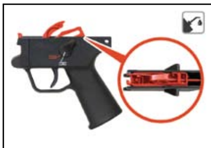
Fig. 49 – Lubrication points on pistol grip
