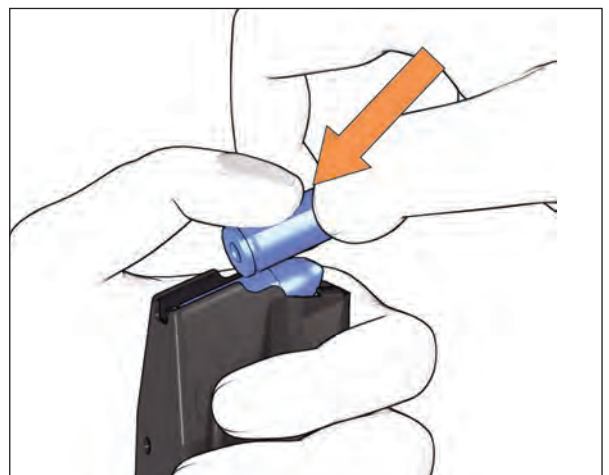
Fig. 29a: Filling the magazine without a loading aid
