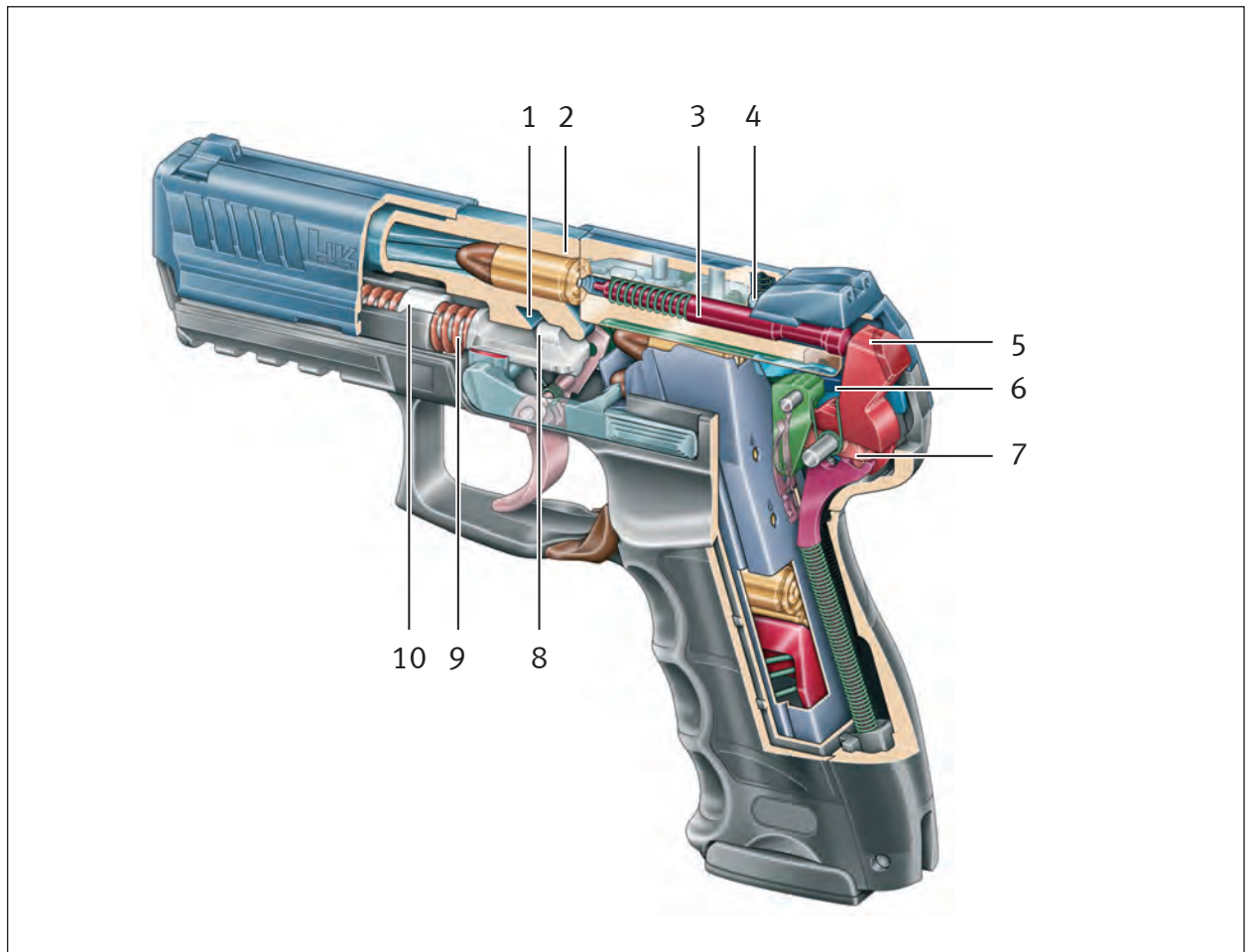
Fig. 13a: CDA trigger variant, cutaway view
