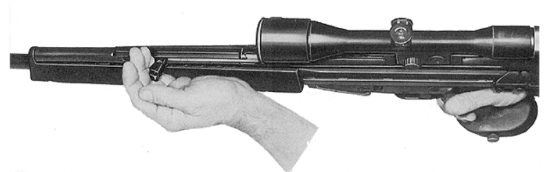
Fig. 19: Pulling back the cocking lever
