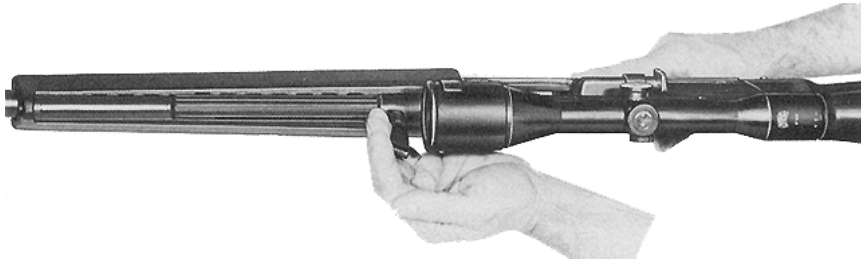
Fig. 20: Releasing the cocking lever to snap forward
