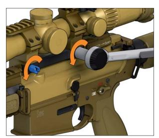
Fig. 56a: Disassembling the 3-20 x 50 telescopic sight
