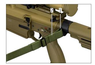
Fig. 33c: Attaching the carrying sling
