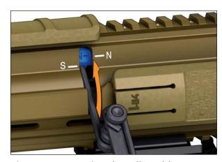
*Fig. 37a:* Rotating the adjustable gas nozzle
