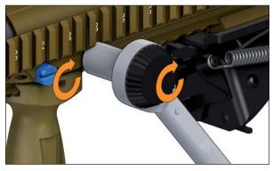
Fig. 67a: Tightening locking screws for handquard
