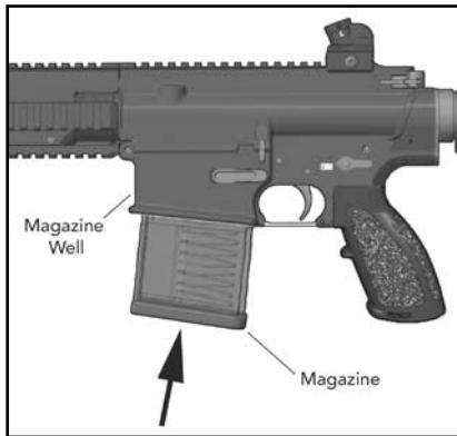
Fig.17 – Inserting Magazine into the Rifle
