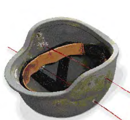
Kevlar helmet penetration at 200 meters. The same 4.6 mm cartridge easily passes through automobile windshields with minimal deflection.
