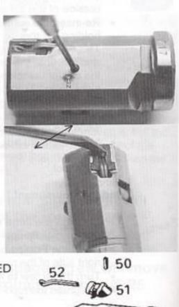
front of the spring against a hard surface and push until the spring seats in the extractor.
